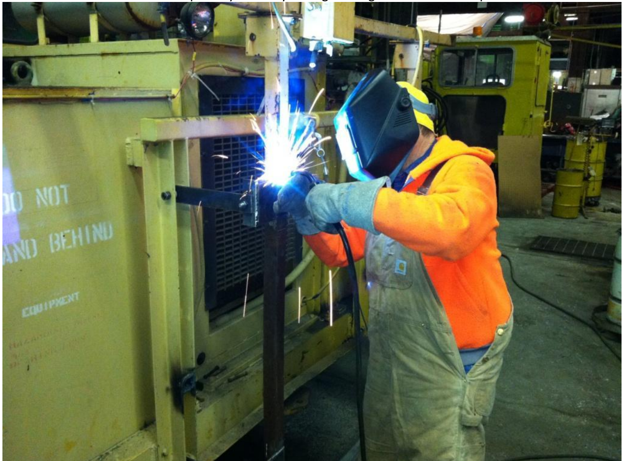
Cliff welds the support bracket for the light receiving stanchion for the surfacing system on the new-old tamper
